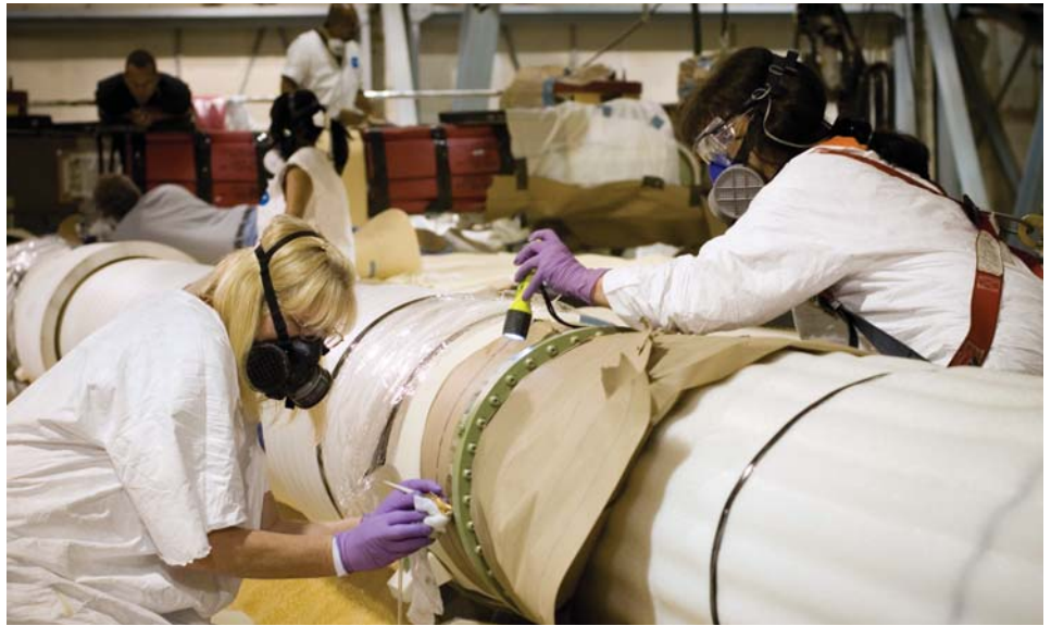
Technicians Judy Atilano (left) and Kathy Wakefield spray primer on an ET-130 LO2 feedline flange.
