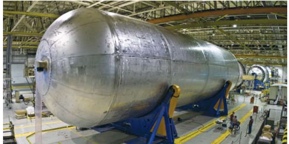
ET-134 will be the first tank to fly using Friction Stir Welding on all of its barrel panels.
