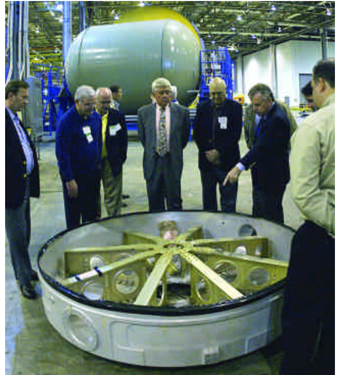
K-1 Program Manager Bob Simms points out to RpK partners a component of the first stage Liquid Oxygen Retention Tank. Michoud work will also include the fabrication, final assembly and integration of several tanks and sub-assemblies.
