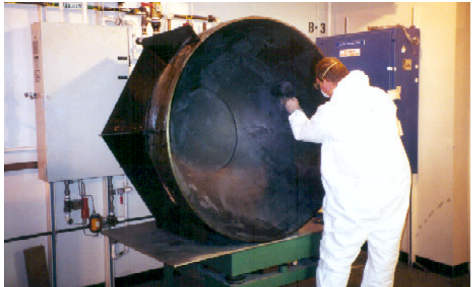
Technician examines a composite tool for making X-34 composite domes.
