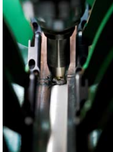
Friction Stir Welding joins two barrel panels using friction and applied pressure.
